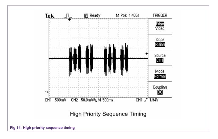
We can see that the high priority sequence has a little more delay between the 3<sup>rd</sup> and 4<sup>th</sup> notes of the sequence, and an even longer delay between the repeating 5 note sequence. This is per the IEC60601-1-8 temporal specifications. Fig 15 shows the medium priority sequence timing.
