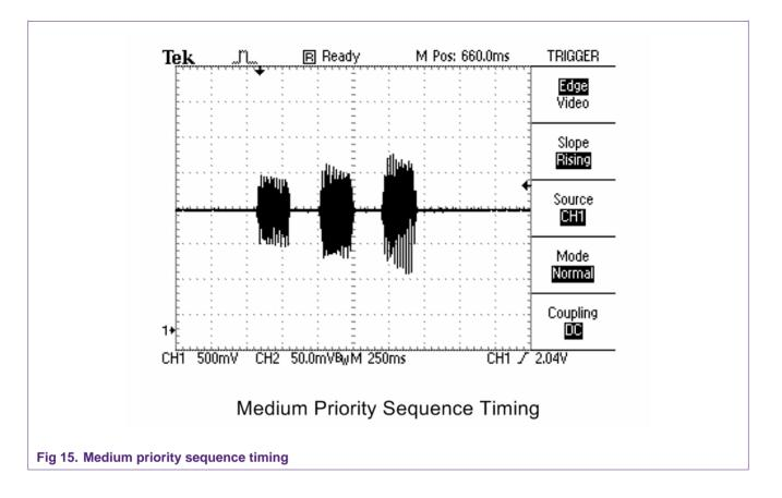
We can see that the medium priority sequence only has three notes and the spacing between the notes is greater than the spacing of the first three notes in the high priority sequence. This is also in compliance with the IEC60601-1-8 specification.
