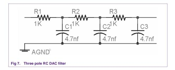
If this is not going to a high impedance input, or if this signal is fed externally, a buffer is recommended.
