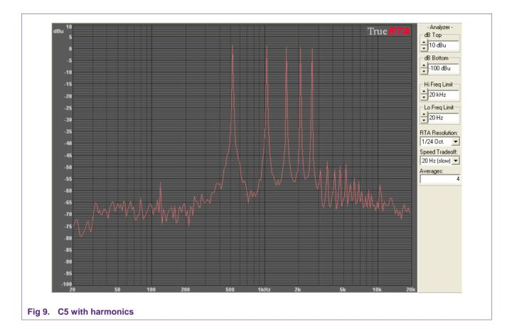
As you can see, the spectrum of the C5 tone with harmonics also has good signal to noise ratios and low distortion while keeping the amplitude of the fundamental and harmonics within a couple of dB.
